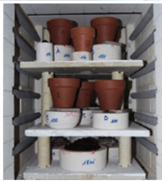
04. The mould is then placed in a kiln with a temperature between 800 and 900 degrees Celsius (1472 - 1652 F). The mould is gradually cooled to avoid thermal shocks.
