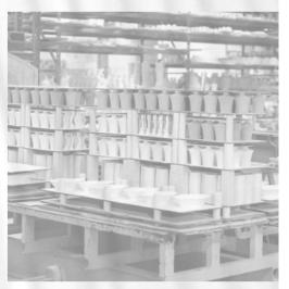
**05.** Drying // It is the time during which the room is stored in the restroom to evacuate naturally its moisture.
