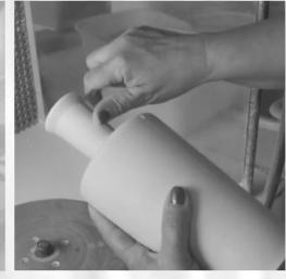
**04. Finishing** // It enables to remove the «seams» on the items caused by the splitting of the mould and to eliminate any other kind of flaws. A steel blade and then mild abrasive are used to polish the object. A wet paintbrush and a sponge are then used for the finishing touch.
